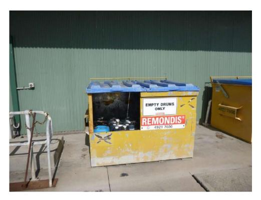
Photo 11 Empty oil and lubricant drums stored within a solid waste bin (not bunded)
